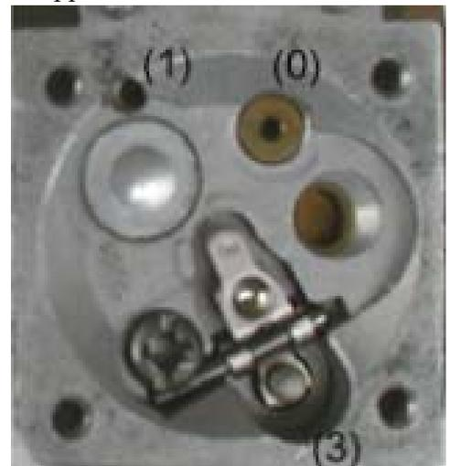
**Figure 9. WA363 Lower chamber with diaphragm removed.**
