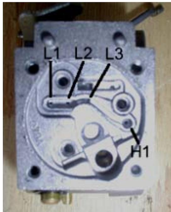
**Figure 11.** WA229 Lower chamber with plate removed.
