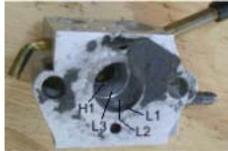
**Figure 12. WT363 Venturi view of fuel metering ports.**
