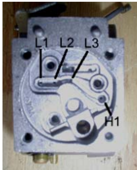
Figure 11. WA229 Lower chamber with plate removed.
