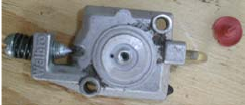
Figure 5. WT363 top plate with check valve removed.
