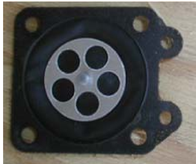
Figure 13. Thick gasket could be between the body & diaphragm as shown here, but not always.
