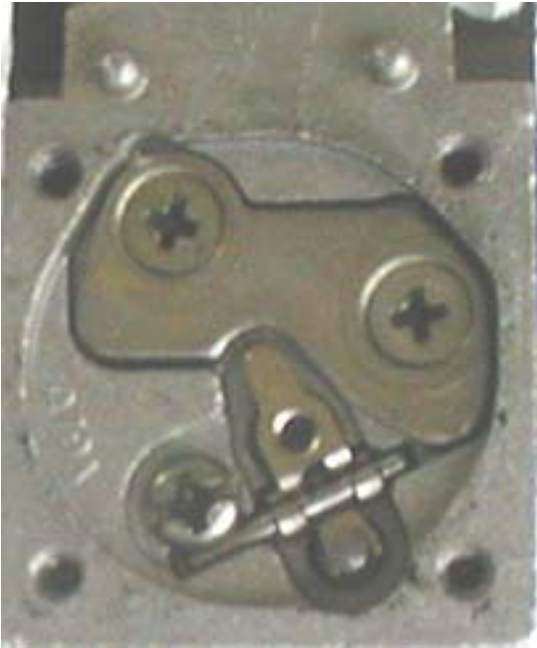
Figure 10. WA229 Lower chamber with diaphragm removed.
