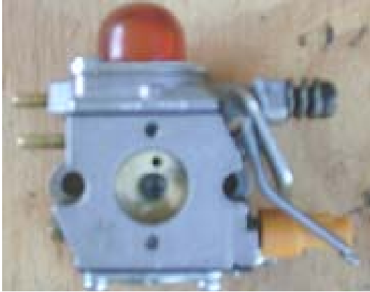
Figure 2. WA229 viewed from engine side.
